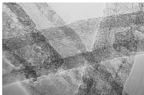
Fig. 5. A high-resolution TEM image of the carbon nanotubes prepared by the template technique.
